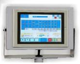
Operator control of is through a touch screen. This enables station selection and output speed, error location and further run information.
